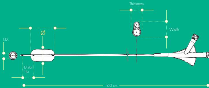
Ø: Diameter I.D.: Internal Diameter O.D.: Outer Diameter L: Length
